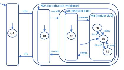
The structure of the above nested state transition system can then be directly taken and translated into the control-flow structure of the program implementation:
